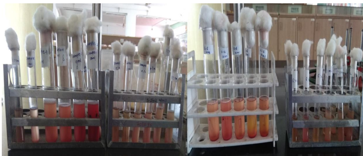
Positive tubes with acid and gas production
