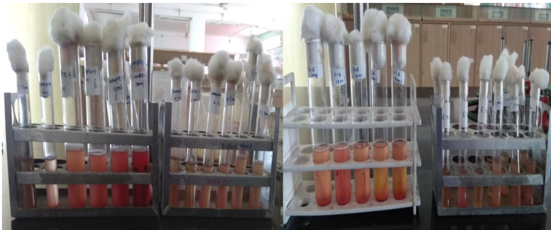
Positive tubes with acid and gas production
